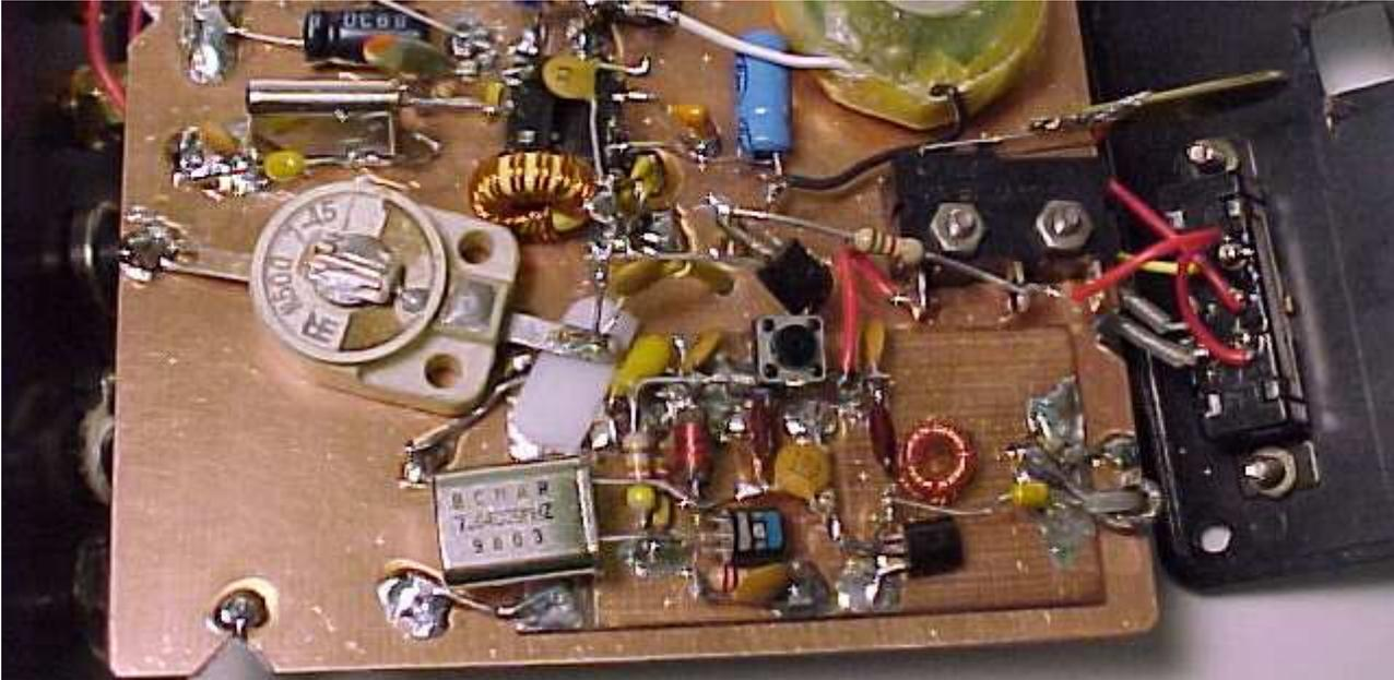
Start with a plain copper-clad board. Glue ICs down with the leads sticking up in the air. Then solder to them
