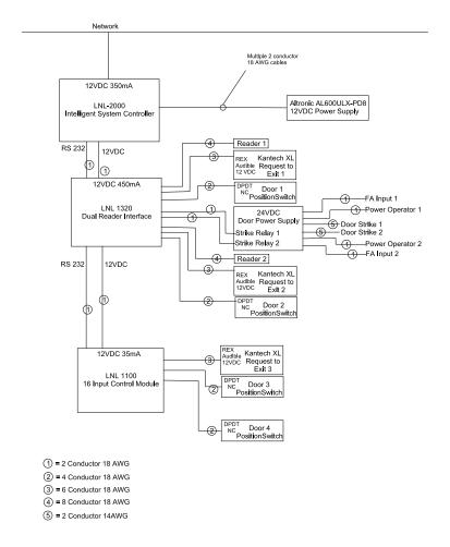
B. See attached installation schematics, also available from FOM Access Control Shop Supervisor:
