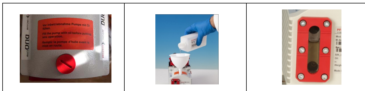
Figure 11 - Rotary pump oil fill
