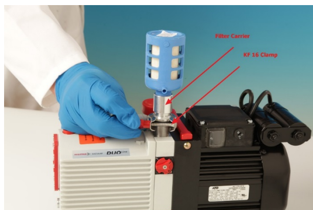
Figure 12 - Rotary pump – oil filter connection
