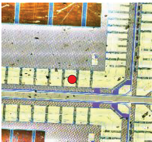
A - Microspot Spot: 1 \mu\text{m} \times 1 \mu\text{m} - Power: 10 mW Power Density: 10 mW/ \mu\text{m}^2
