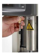
The tweezers with grid are subsequently lifted into the climate chamber by selecting the 'Start Process' button in the User Interface, or alternatively, use the foot pedal switch. The environmental and process parameters (i.e. temperature, humidity, number of blots etc) can now be set as described in:
