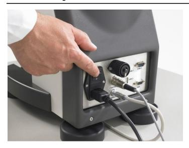
After activation of the hard lock switch the embedded PC with Linux operating system is automatically starting up. The Vitrobot User Interface page will appear after a few seconds.
