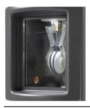
Note After a maximum of 16 blottings, the filter papers must be replaced. The UI displays the message: 'Replace Blotpapers'.
