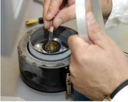
After the grids have been transferred into the grid box, they are sealed with a special screw and usually stored into a somewhat larger dewar for liquid nitrogen prior to the transfer into a cryo holder and subsequently a TEM or SEM.
