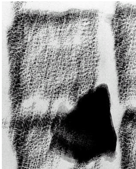
Misaligned diffraction shift pivot point.
