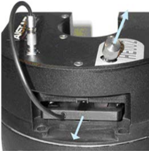
Figure 3.4.1 Removing the probe holder from the AFM measuring head HE002
