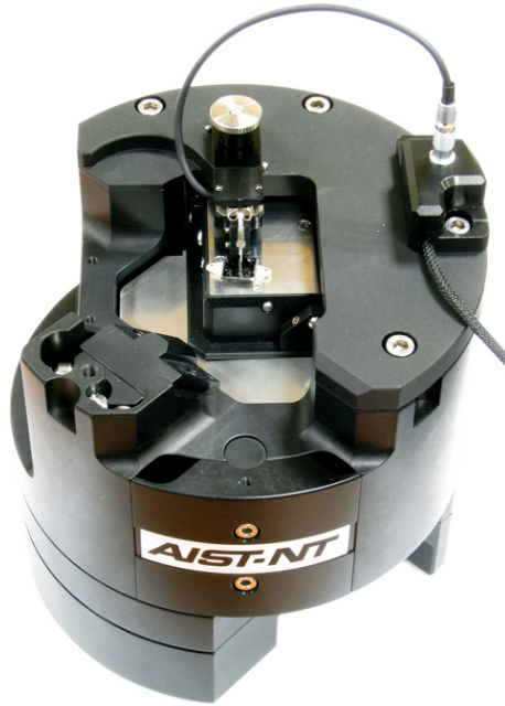
Figure 7.4.1 SmartSPM setup for measurements with quartz tuning-fork
