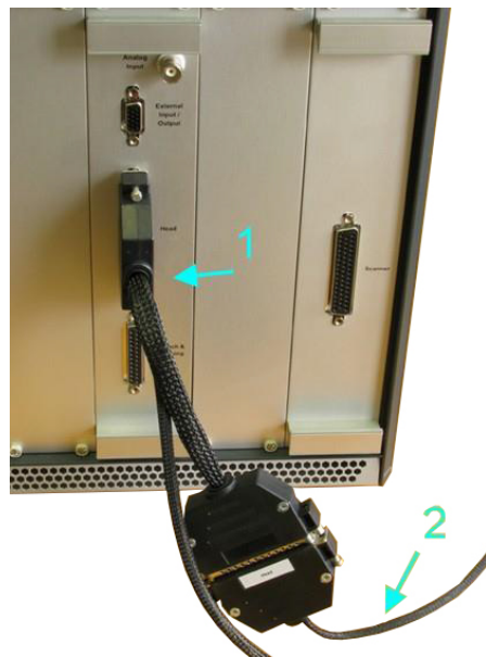
Figure 7.1.3 Cable connection of the conductive unit to the controller.
