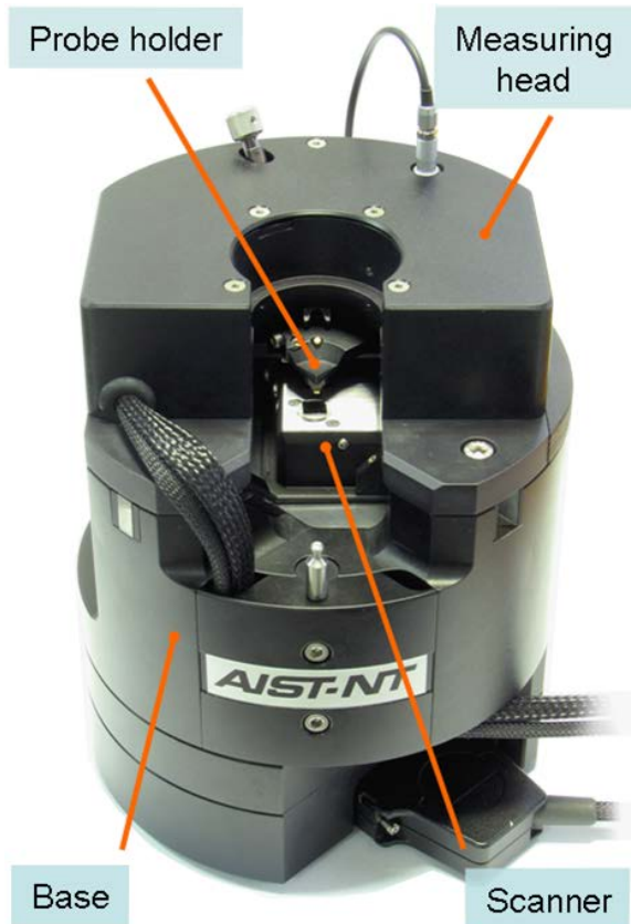
Figure 1.1.1 SmartSPM main parts
