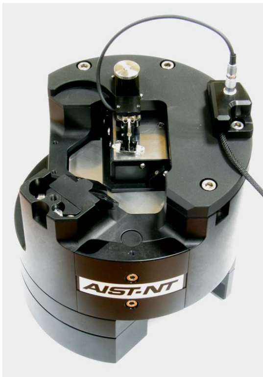
Figure 7.4.5 SmartSPM with the accessories mounted for working with the quartz oscillator.
