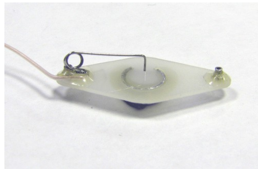
The sample holder with spring for electrical contact to the
