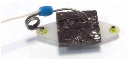
Figure 7.2.2 A piece of HOPG installed on the sample holder with spring clip
