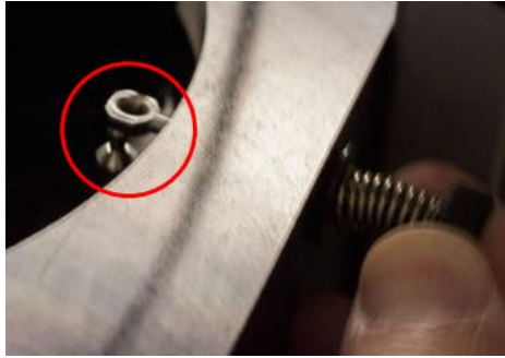
Hook the bolt by screw.
