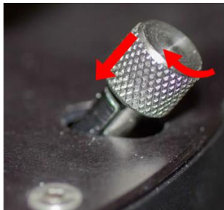
Down position of the latch
