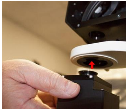
Place the objective scanner into the flange
