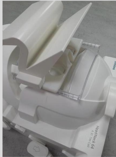
Lens holder for Siemens 64 channel head coil
