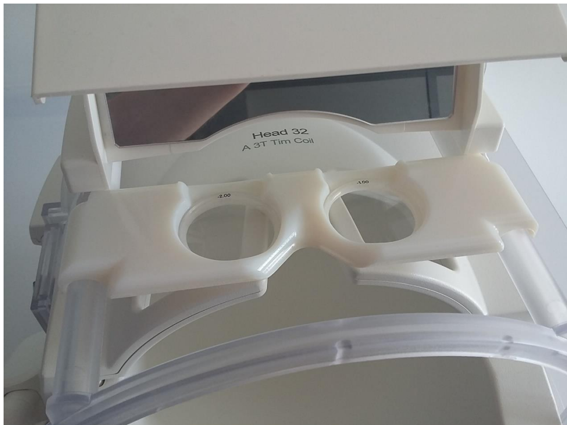
Figure 4. Lens fitted into the lens holder.
