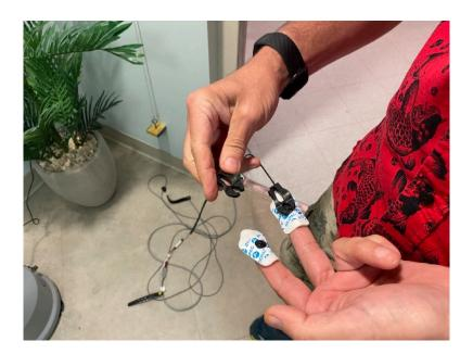
To connect the photoplethysmogram, connect a single finger contact like this:
