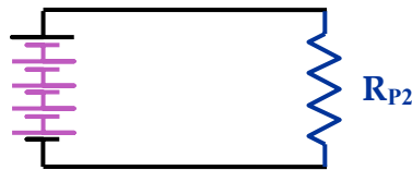
Fig. 27. Final simplified circuit. R_{s1} and R_{s2} are have been combined in parallel. The current in the resistor can now be found by simple application of Ohm’s law.
