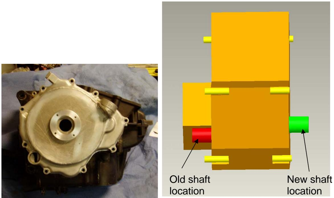
Figure 3: Shaft Relocation
