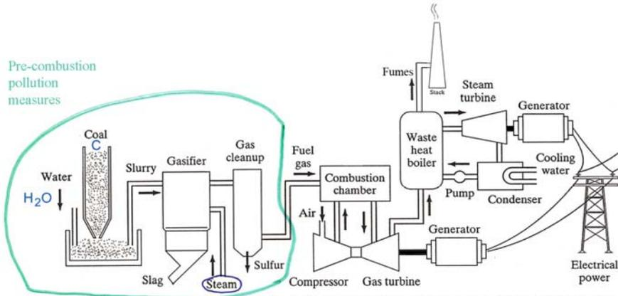
FIGURE 7.29 Integrated gasification combined cycle. Gasified coal fuels an efficient gas turbine; waste heat from the gas turbine powers a steam cycle.
