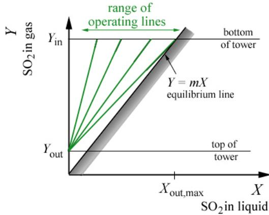
Since the amount of liquid used ( $L$ ) is free to be chosen, we can consider a series of different operating lines, one for every slope  $(1+c)L/V$  considered. In order to stay on the upper side of the equilibrium curve, however, there exists a minimum acceptable slope, and there is therefore a minimum value of the liquid mass flow,  $L_{\text{min}}$ , that must be used.
