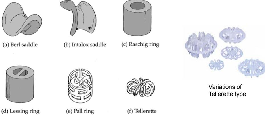
These elements are designed to create tortuous flow paths in order to maximize contact between gas and liquid.
