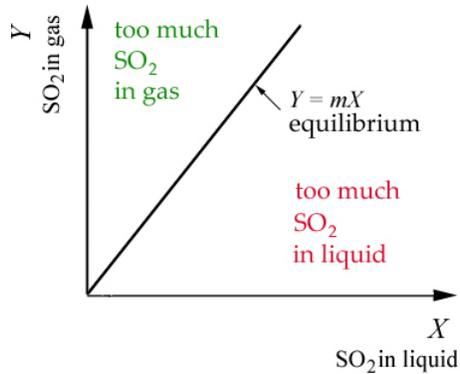
At the temperature and pressure common in the operation of scrubbers, SO<sub>2</sub> equilibrium is achieved when the gas fraction is about 36 times the liquid fraction. Therefore, a practical value is
