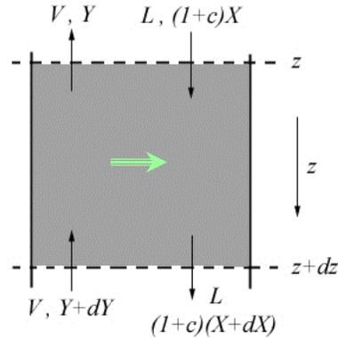
The steady-state budgets express that the rate at which the amount in each phase (gas or liquid) enters the slice is equal to the rate at which it exits plus or minus the amount exchanged with the other phase:
