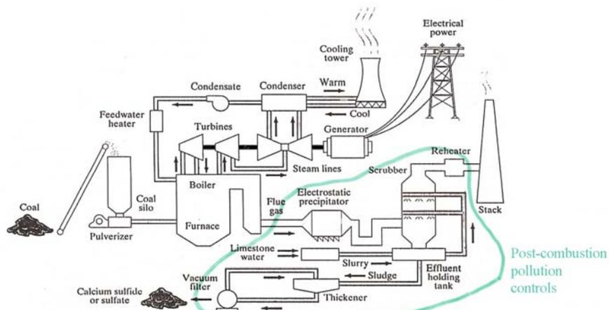
FIGURE 7.27. Typical modern coal-fired power plant using an electrostatic precipitator for particulate control and a limestone-based  $\text{SO}_2$  scrubber. A cooling tower is shown for thermal pollution control.
