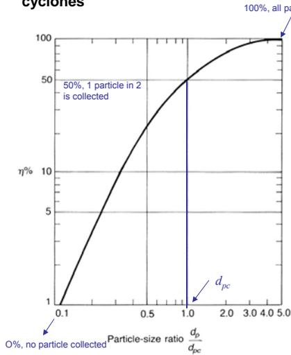
Lapple then developed a general curve for standard conventional cyclones to predict the collection efficiency for any particle size (see side figure).
