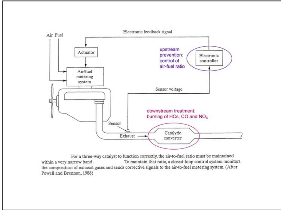
A three-way catalytic converter performs three simultaneous tasks:
