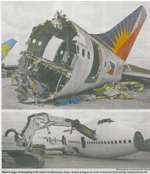
Planes at stages of dismantling at the airport in Châteauneuf, France. It takes as long as six weeks to break down the average commercial aircraft. Photograph by Jean-Pierre Pélissier/Reuters
