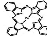
Zinc-Phthalocyanine \lambda_{\text{max}} 671 nm ( \epsilon 2.7 \times 10^4 \text{M}^{-1}\text{cm}^{-1} )
