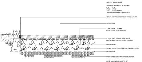
NOTE: UNDERDRAIN & DEPTH OF SUB-BASE MATERIALS VARIES ACCORDING TO SITE SPECIFIC CONDITIONS.
