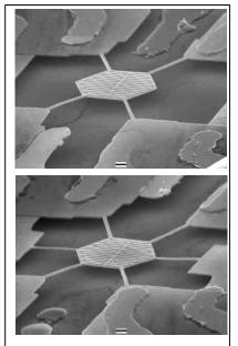
**Figure 1 a,b.** Suspended four- and six- conductor devices.
